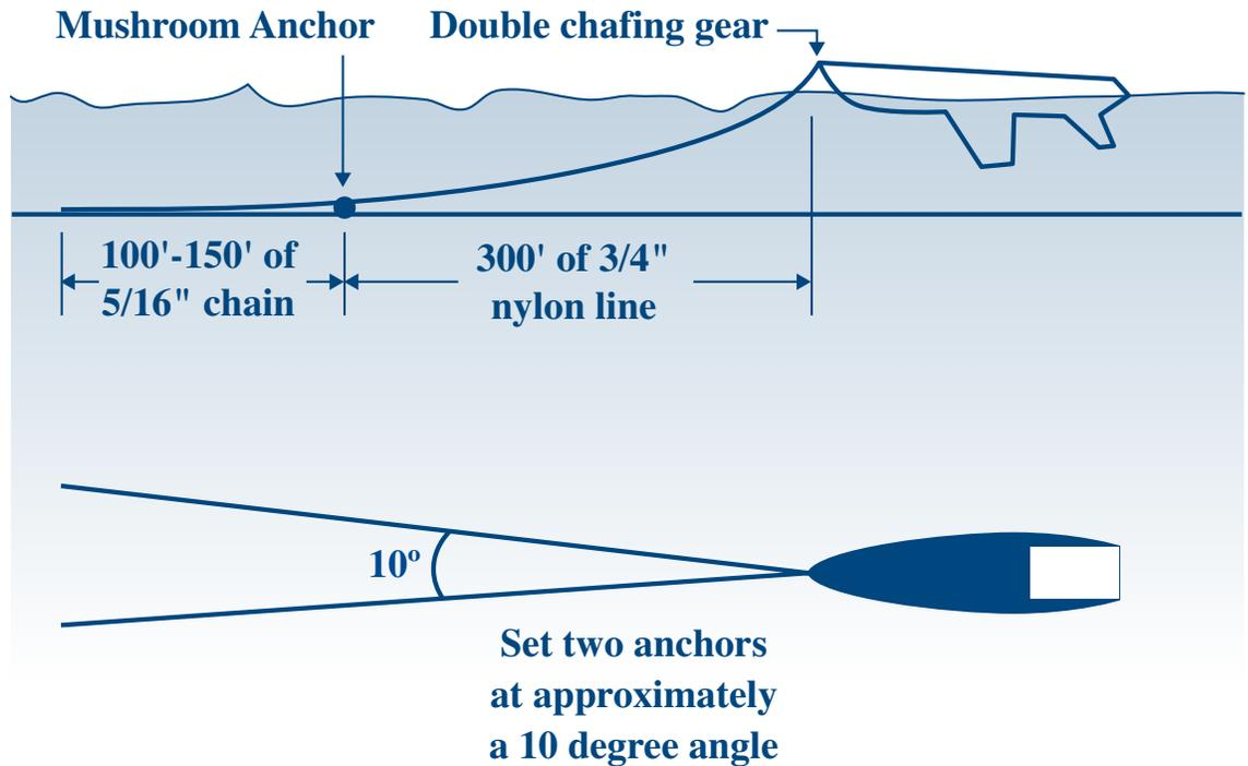
**Galveston Bay Anchor System** – Set two bruce or CQR anchors on 100' to 150' 5/16" chain and 300 feet of three strand nylon line with a 50–100 pound mushroom anchor shackled on the boat end of the chain, attached to the boat with 3/4" nylon bridle with double chafing gear.
