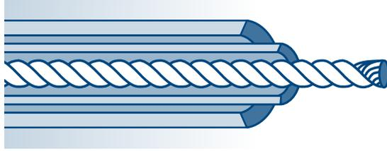
For a super system, if your chocks are large enough, fit a second, larger-diameter hose around another hose that fits snugly to the line. Drill holes in both hoses, and use cord to tie them securely to the line. In a pinch, you can use a single hose.
