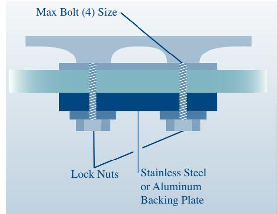
**Reinforced and properly backed cleat: note the washers and the backing plate. These are essential in a severe storm, and a good idea in quieter times as well.**
